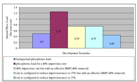
Figure 7.22 Phosphorus Loads under Different Land Uses and BMPs
