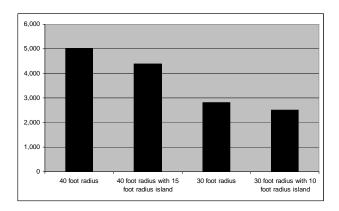
Figure 7.34 Comparing Impervious Cover of Cul-de-sac Alternatives
