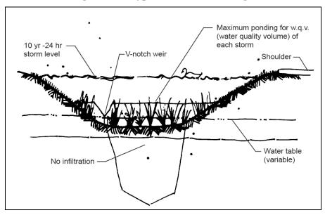
Figure 7.17 Typical Wet Swale Design
